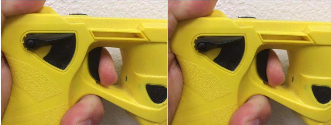
Trigger pull necessary to deploy cartridge
